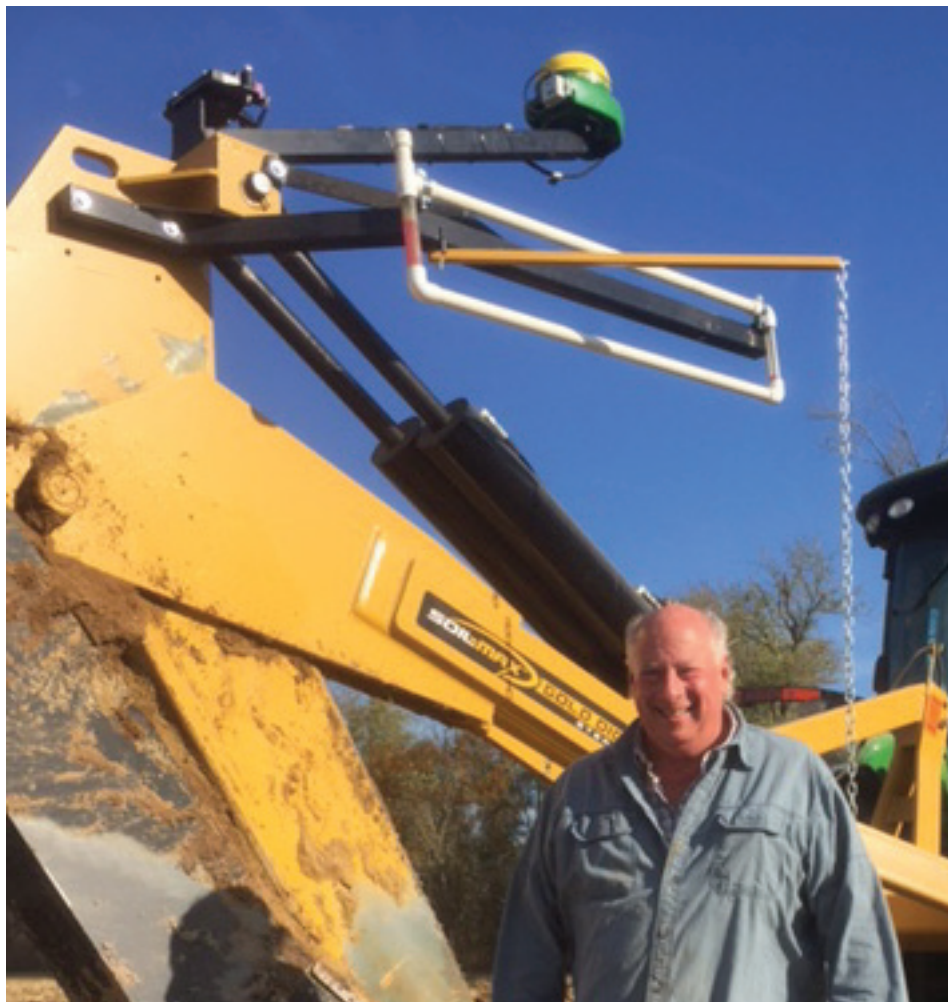
Bobby Boggess and his tile plow, which is guided by a John Deere StarFire 3000 Receiver, receiving its RTK corrections wirelessly via Intuicom’s RTK Bridge-X Bluetooth Receiver.
