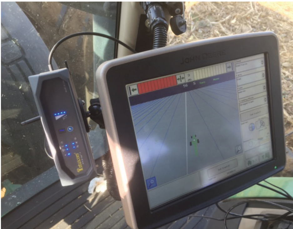
Connected along side of Bobby Boggess' Intellislope Guidance System, the RTK Bridge-X front panel displays real-time cellular signal strength, as well as status lights for Power, Wi-Fi Signal, Bluetooth Connectivity, Ethernet, GPS, NTRIP Server, and Data/Corrections.
