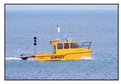
"A survey vessel with the RTK Bridge installed served as our base, capturing and rebroadcasting RTK network corrections to our second vessel equipped with a rover."
