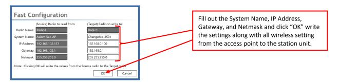
Once the radio has the settings written to it, it will pop up under the Broadband Units column and display as a station with the S icon on it.
