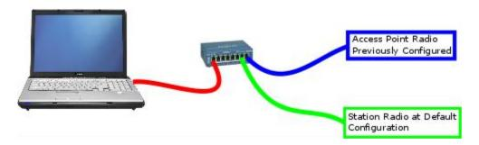
By connecting up both radios to the switch you will be able to see both in the BroadBandPro<sup>™</sup> 5 software, and take advantage of the drag and drop feature that will allow you to program all the wireless settings with two simple steps.
