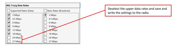
After you have written the settings to both access point and station radio, look at the "Link Stats" tab and monitor the connection and watch the CCQ. It should climb up to the 90 to 100 percent range. This may take a few minutes for the reading to stabilize and climb to its maximum value. If the CCQ value does not come up into the 90-100 percent range, try deselecting one more data rate on both radios and see if that gets it up into the desired range.
