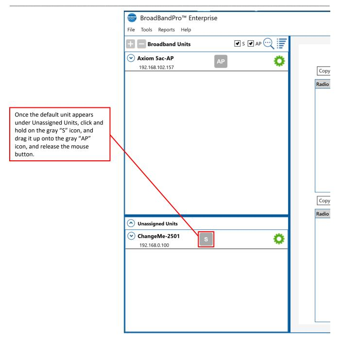
**NOTE:** The Radio is dragged and dropped onto the radio that you want to connect it with. This is done this way so that users can drag multiple radios to the appropriate radio they want to connect it with. An example is if you are using a Dual unit with two radios in it, you will need to drag the radio in the station to the appropriate radio in the Dual where you want it to connect, or vice versa.
