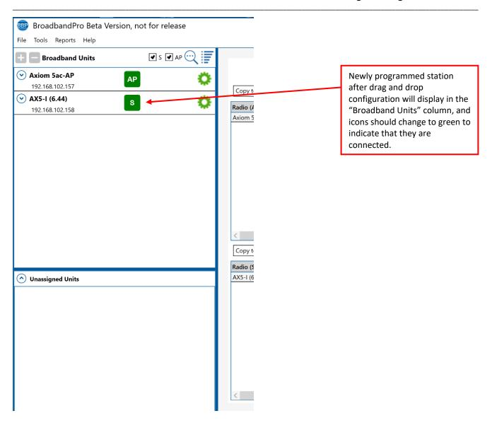
If you have a large deployment with access point radios that will have multiple stations connected to each unit, the drag and drop feature of BroadBandPro $^{\text{TM}}$  5 software will save a considerable amount of time with programming the radios.
