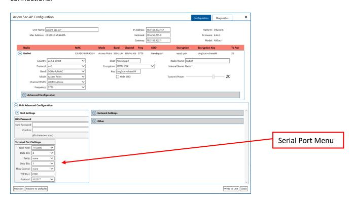
You will need to set the Baud Rate, Data Bits, Parity, Stop Bit, and flow control to match the device you plug into the serial port. You can also change the TCP port if needed. Typically the Protocol is set to raw, however, rfc2217 setting is also available if needed.
