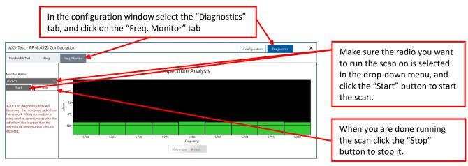
**NOTE:** Typical noise floor is around -115dB – Between -100dB and -120dB or weaker. **Signal Strength** is typically optimized by aligning the radios and adjusting the Tx power on the radio to get as close to the -50dB reading as possible.
