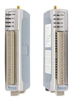
The Intuicom VUE-24-IO Wireless I/O and Gateway is a multiple I/O device that extends communications to equipment, sensors and actuators in local, remote, or difficult to reach locations. Designed with a long range, license-free wireless transceiver, the VUE-24-IO can provide IP-based mesh networking across sprawling environments typical of industrial applications.
