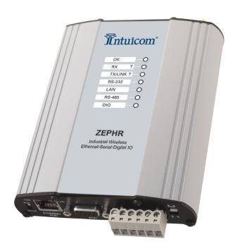
The Intuicom ZEPHR-2 wireless Ethernet modem is a robust, inexpensive, license-free wireless 802.11 standards-compliant transceiver capable of high-bandwidth communications. Operating at 2.4GHz and up to 630 mW, the Intuicom ZEPHR-2 is optimized for data rates of up to 108 Mbps, providing robust long-distance and secure two-way wireless communications in challenging environments typical of industrial monitoring and control applications.
