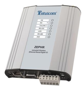
The Intuicom ZEPHR-5 wireless Ethernet modem is a robust, inexpensive, license-free wireless 802.11 standards-compliant transceiver capable of highbandwidth communications. Operating at 5.8GHz and up to 630 mW, the Intuicom ZEPHR-5 is optimized for data rates of up to 108 Mbps, providing robust long-distance and secure two-way wireless communications in challenging environments typical of industrial monitoring and control applications.
